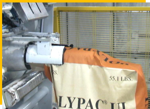
Bag during filling operation Dettaglio saldatura
